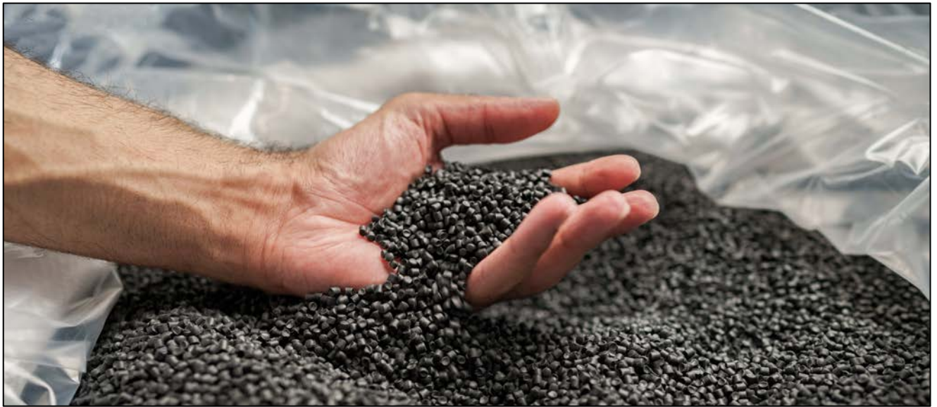
Caption: Exemplary rPET ReCompound after the recycling process of the CF PET carrier rolls.
