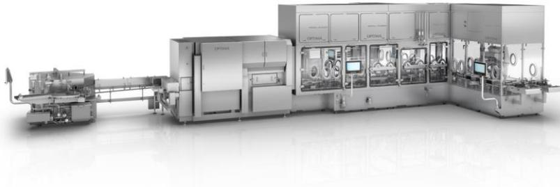
Optima has worked with numerous pharmaceutical companies to modify filling and closing systems under construction and design new ones in record time. Optima Pharma's vaccine filling and closing lines are capable of washing, sterilizing, filling, and closing vials under an isolator. (Source: Optima)
