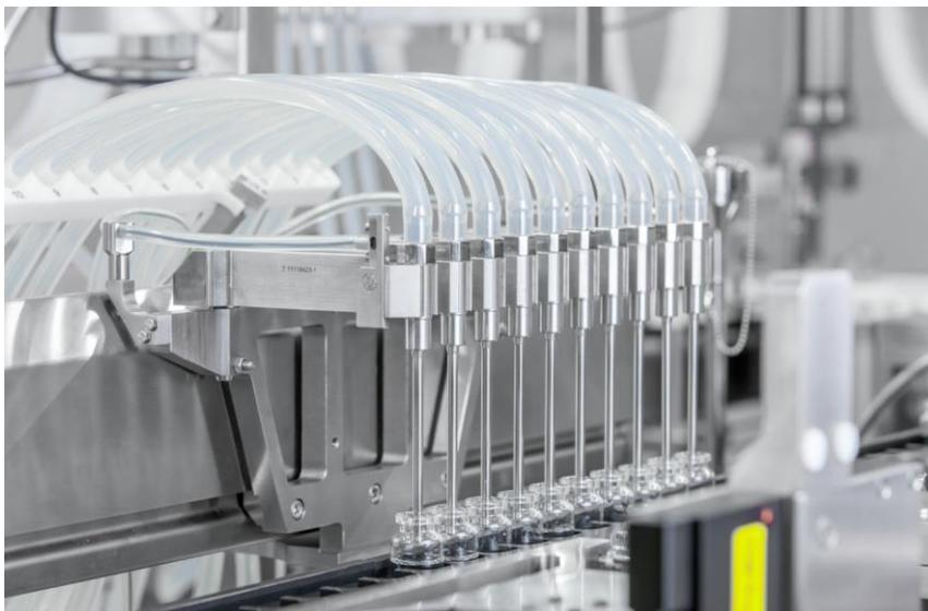
The vaccine is dosed multi-dose into the vials. Different filling technologies suited to different liquids ensure the greatest possible flexibility when filling different pharmaceuticals. (Source: Optima)
