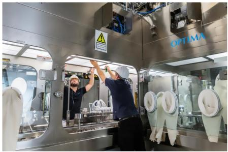
At Optima Pharma in Schwaebisch Hall, the system components – consisting of filling and closing equipment and isolator – come together and are commissioned under real-life conditions. This means a considerable time saving before production starts on the customer's premises. (Source: Optima).
