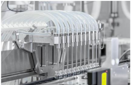
The vaccine is dosed multi-digit into the vials. Different filling technologies suited to different liquids ensure the greatest possible flexibility when filling different pharmaceuticals. (Source: Optima)
